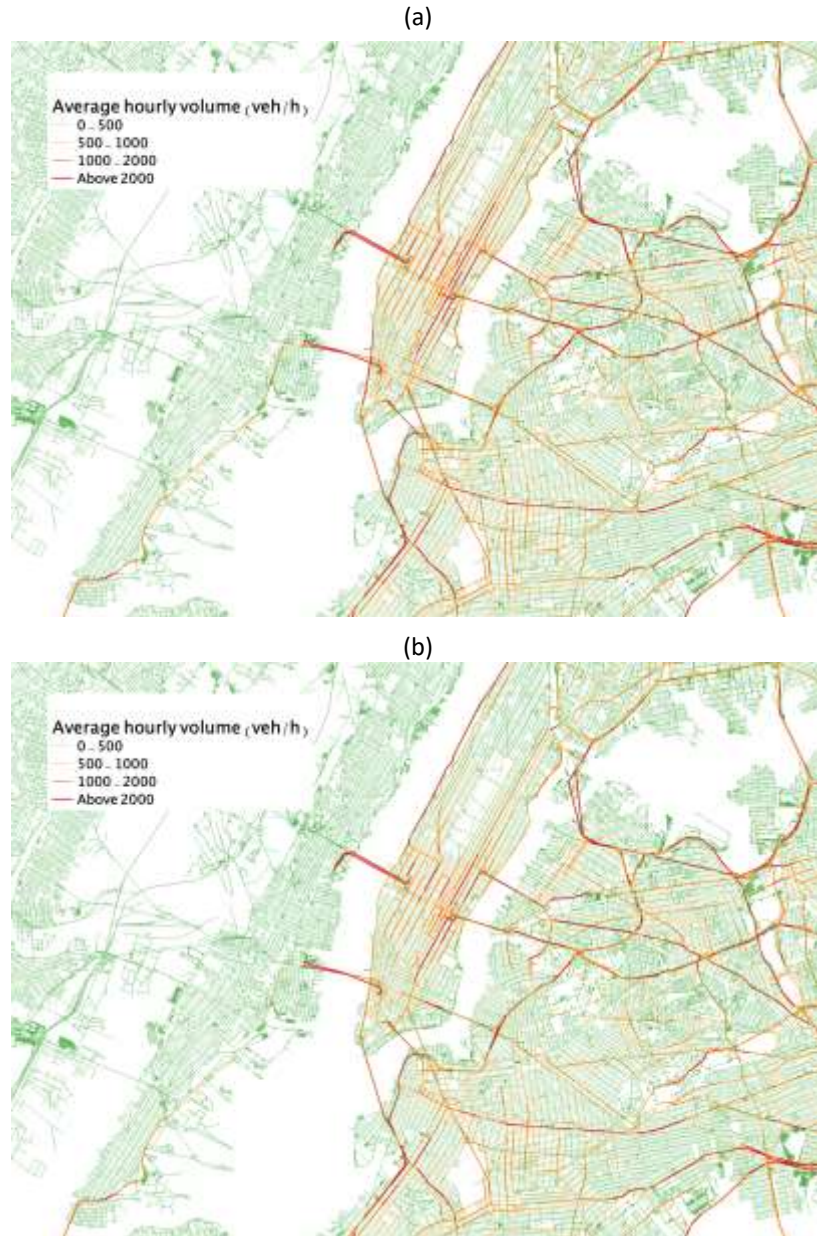
Figure 33. Average hourly volume distribution (a) before congestion pricing and (b) under Schema 2.
