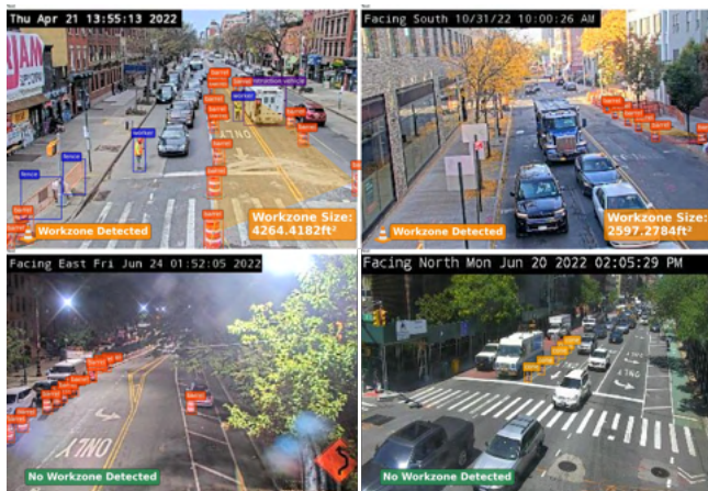
Fig. 5. Output of work zone detection, inference, and area estimation. The top two images highlight detected work zones in orange, with estimated sizes at the bottom right. The bottom two images show correct detection of non-work zones that contain work zone equipment.
