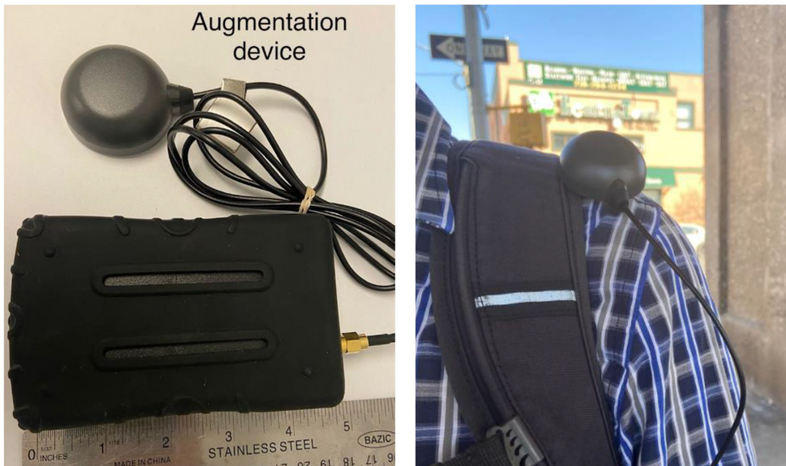
Figure 14. Augmentation Device and Antenna Position
